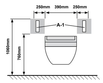
Temporarily place the remote control in the position determined in and confirm the signal reception of A-1.
